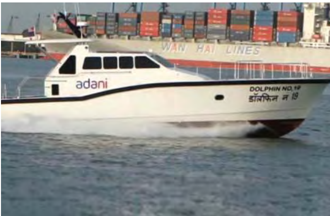
16.7m Patrol boat, designed by Icarus Marine Many vessel builders use proven designs, to be confident that finished products will meet contracted speed requirements. In the absence of a proven design it is common practice to test the hull of the vessel at a ship model test basin. Icarus Marine in Cape Town uses a 100m model test tank at Stellenbosch University, as well as computational fluid dynamics (CFD) analysis, to ensure predictable performance of full-scale, original designs.
