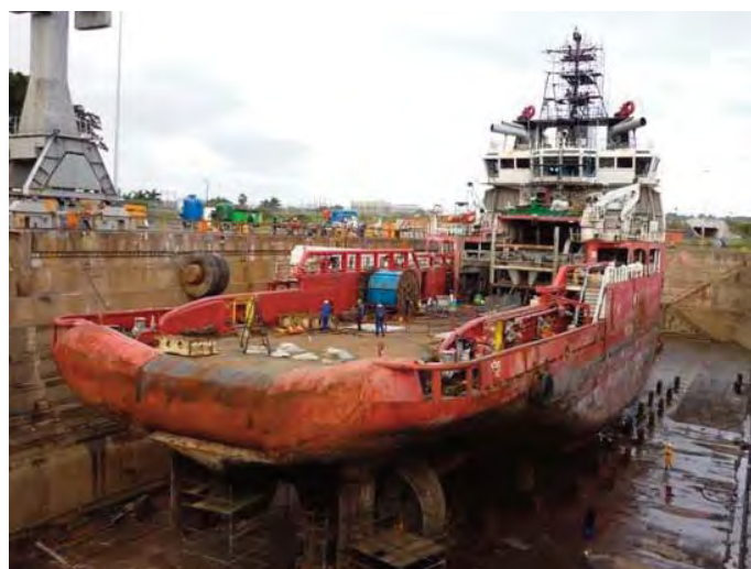
Electrical refit and full powertrain overhaul of the fire-damaged offshore tug Subhiksha, by Southern African Shipyards. A complete overhaul to the main engine and crankshaft; thrusters, propellers and main shaft. Replacement of all electrical items, including over 15km of wiring.
