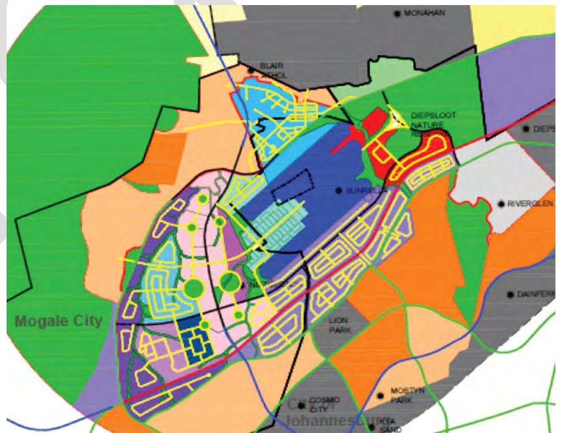
Figure 29: Spatial Development Concept Plan indicating the expansion of the airport and the realignment of the PWV 3
