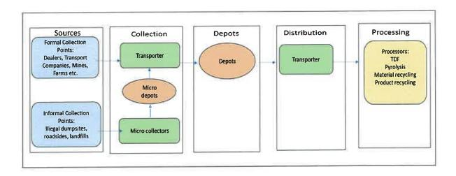
Figure 8: Waste Tyre management process flow
